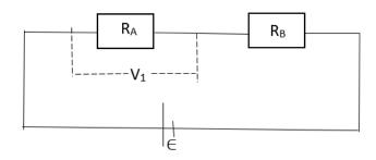
$$V_{1} = IR_{A} \text{ But } I = \frac{\epsilon}{R_{T}} \text{ and } R_{T} = R_{A} + R_{B} = \frac{\rho_{1L}}{A} + \frac{\rho_{2L}}{A} = \frac{L}{A} (\rho_{1} + \rho_{1})$$
