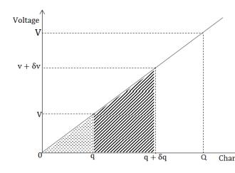
When a small amount of charge  $\delta q$  is transferred from q, then;-
