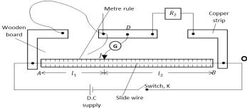
• The diameter of a specimen wire of known length x is measured at different points using a micrometer screw gauge and its mean diameter, d is determined.
