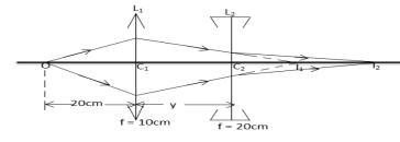
Action of the converging lens,  $U_1 = 20 \text{cm}$ ,  $V_1 = ?? f = 10 \text{cm}$
